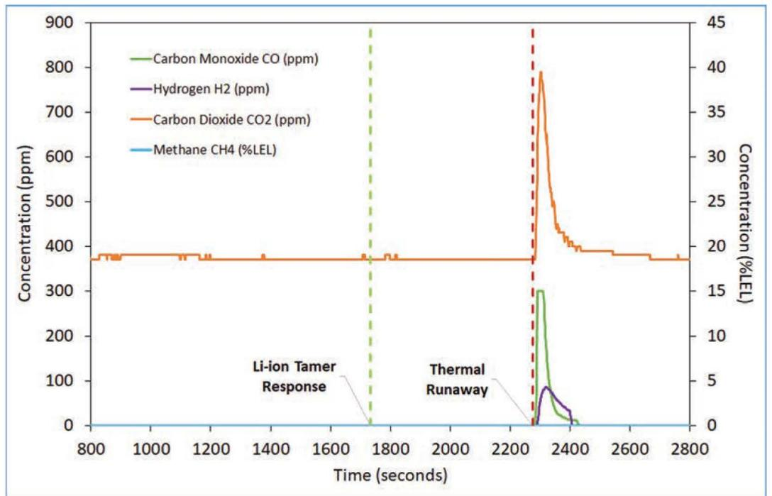
There were no responses from any of the conventional gas detectors during the electrolyte vapour event or prior to thermal runaway.
