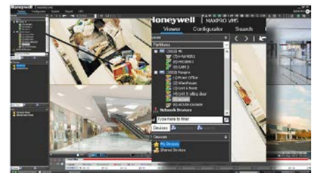
Honeywell's MAXPRO VMS (video management system) controls multiple sources of video subsystems to collect, manage and present video in a clear and concise user interface.
