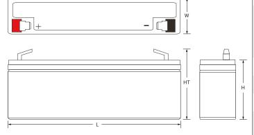
**L:** 7.00 (178) **W:** 1.37 (35) **H**: 2.36 (60) HT: 2.59 (66) Tolerances are +/- 0.04 in. (+/- 1mm) and +/- 0.08 in. (+/- 2mm) for height dimensions. All data subject to change without notice.
